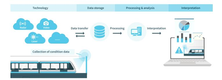
Wayside Train Monitoring Systems (WTMS) are track-bound diagnostic systems that utilize a range of sensors and measurement devices to monitor the condition of passing vehicles in real time (e.g. the condition of pantographs, which are devices that collect electrical power from the overhead line, or the degree of contamination).
